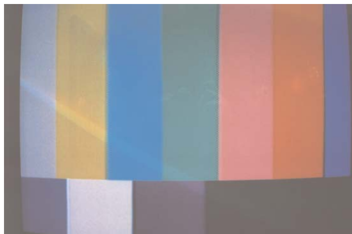
Demodulated 1253.25 MHz VSB signal as displayed on a video monitor, note the lack of video artifacts (except light reflecting from the monitor screen) and broadcast quality picture displayed.
