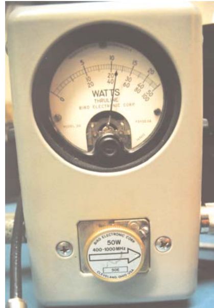
Bird 43 with peak detector on confirming 22 watts peak sync output.
