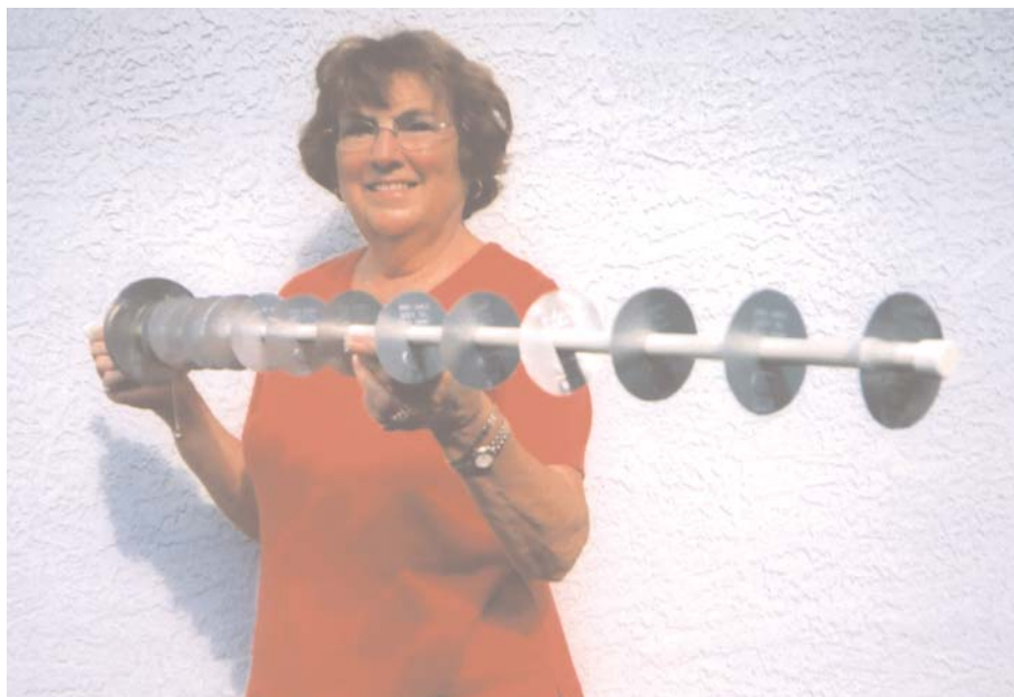
N8LEP, Patty Parker, holding rod & disk antenna for 23 cm ATV usage.
