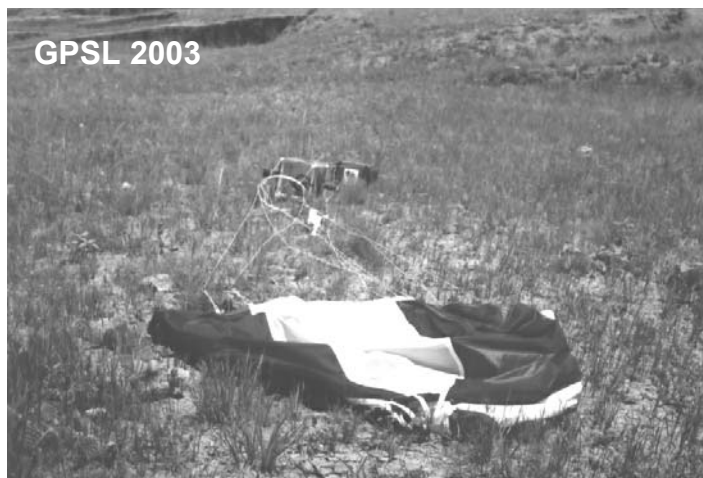
One of the TVNSP near spacecraft after recovery. This near spacecraft carried two balloonsats to 90,000 feet.
