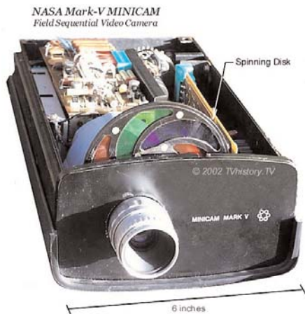
Figure 15 Field Sequential Color Camera used by NASA for Apollo
