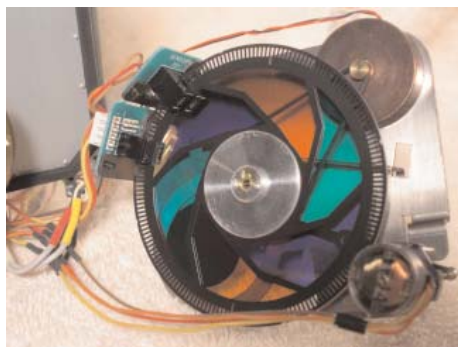
Figure 16B Color Wheel Mechanism (JVC TK-F7100U)
