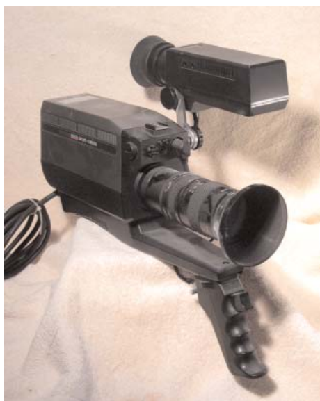
Figure 19A Hitachi GP-5U Single RGB Tube Color Camera (1976)
