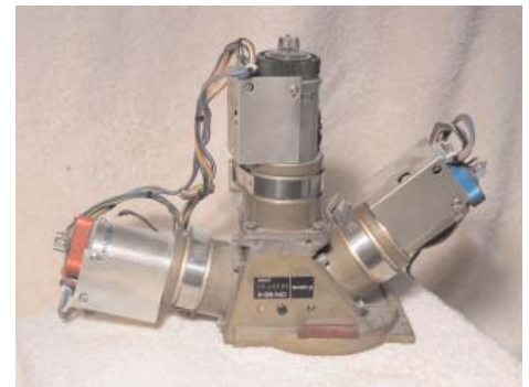
Figure 11 Sealed Prism Block, with three 18mm tubes
