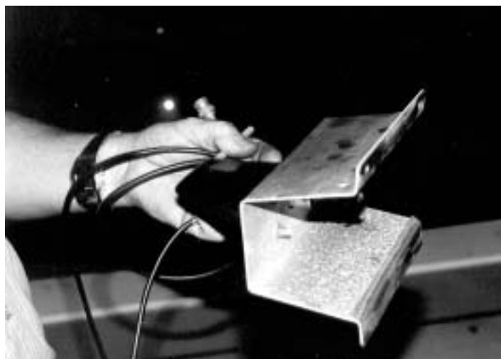
Above and left - Fabricating the 434 MHz helicopter antenna mount for the ATV transmitter.
