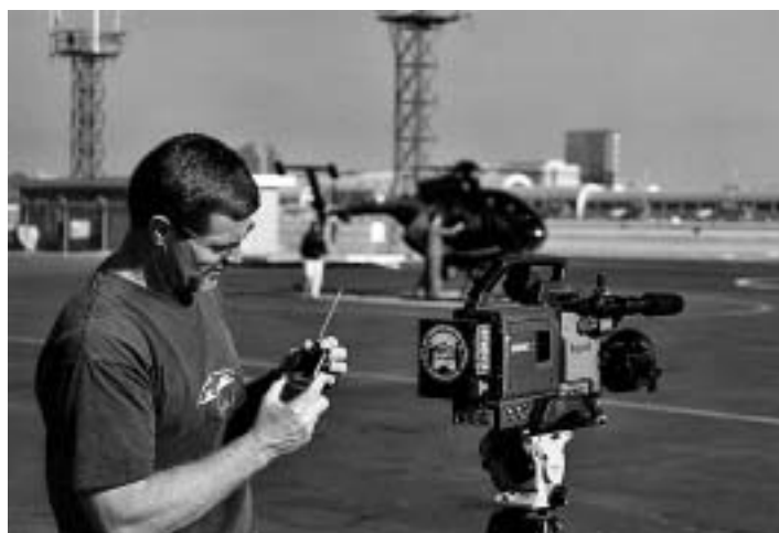
The ICOM R3 tunes in ATV from the helicopter up to 10 miles away simplex.
