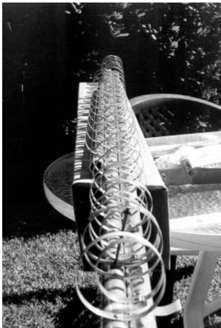
The loop yagi from directive systems is perfect for ATV 1250 MHz repeater reception.
