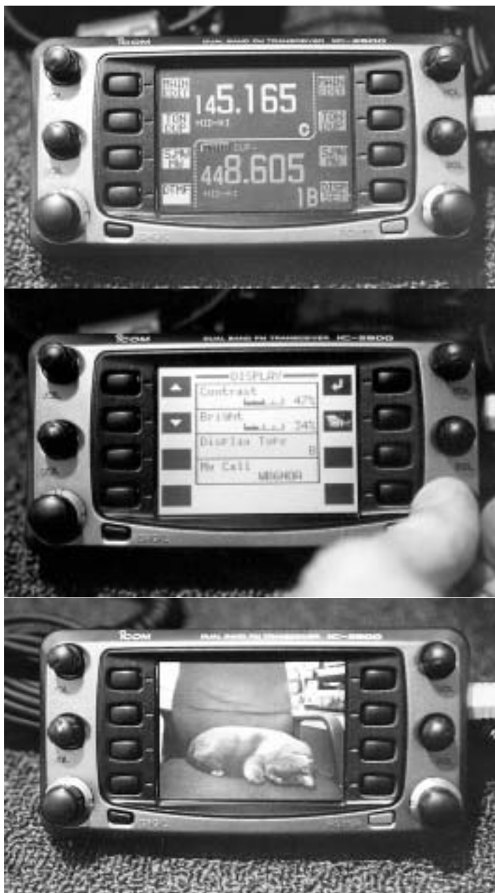
The ICOM 2800 ham radio can display ATV video from the helicopter VCR video output jack.
