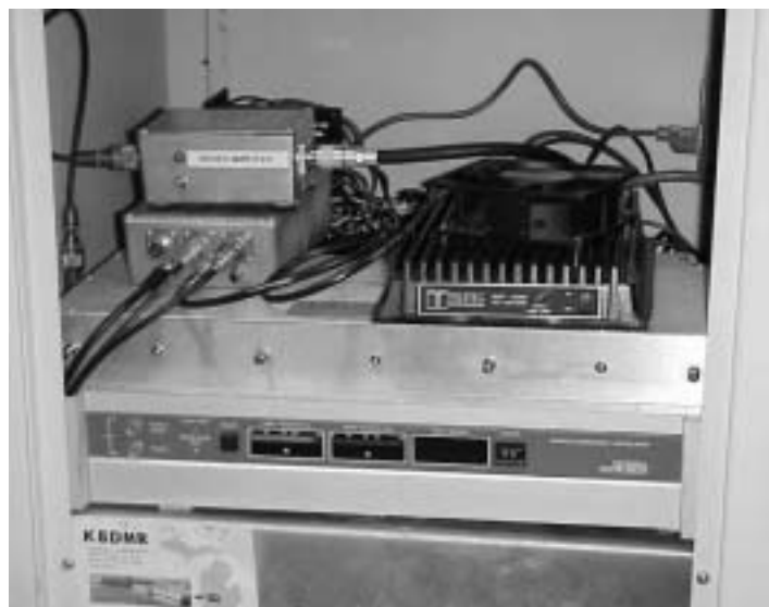
(4) Close-up showing General Instruments exciter and PC Electronics driver amplifier in die-cast box. High power Teltec amp sitting on filter at right. Fans key on with repeater.
