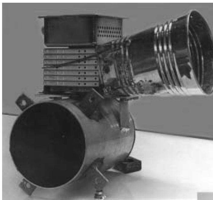
The feed horn with magnetron and air hose adapter mounted.
