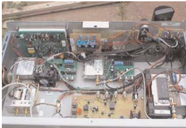
The inside of my general purpose 1.3GHz transceiver
