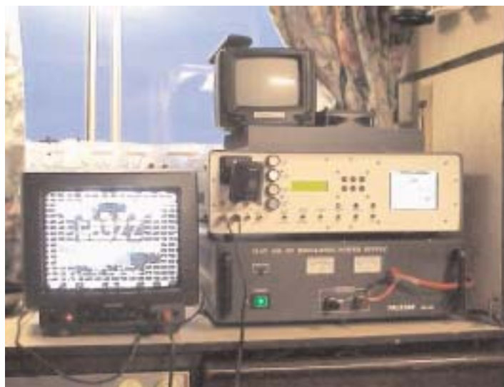
High power 1.3GHz transceiver receiving repeater GB3ZZ at a range of about 25 miles
