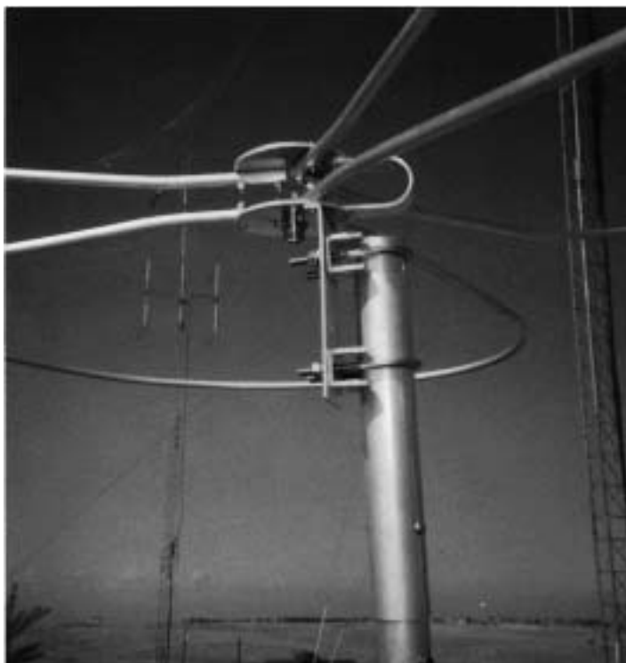
“Big Wheel” closeup showing detail of hub, connector and stub.
