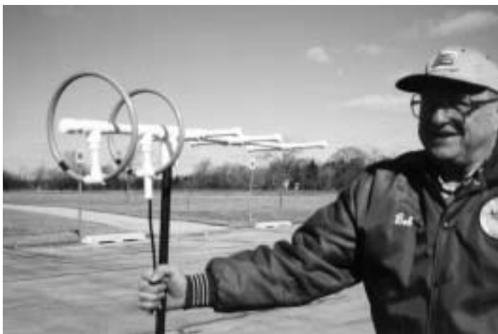
440 Quad Full Wave used on Icon R-3 for distance.
