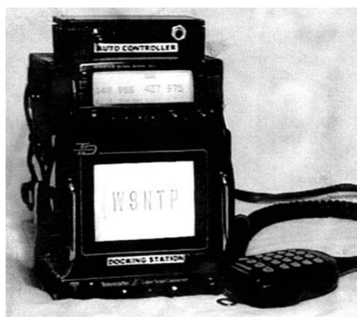
CLOSEUP VIEW OF THE MIR DOCKING STATION USING THE W4HTB CONTROLLER, KENWOOD TM-V7A, LCD DISPLAY AND THE TASCO TSC-70
