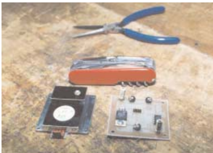
SHF Microwave PS/MOD kit for Gunnplexors under construction by W3HMS. Pliers and Swiss Army Knife are for size comparison
